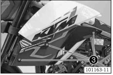
Install and tighten screw ② with the bearing sleeve and rubber sleeve on both sides. Check the fuel tank for tightness.
