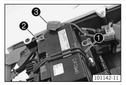
Position the battery in the battery rack.
