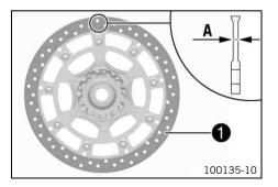
Check the thickness of the brake disc in several places to see if it conforms to measurement ①.
