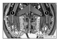
− Turn adjusting screws ● clockwise all the way.
