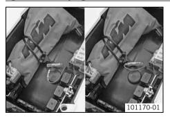
The plug-in connection is located under the seat in front of the fuse box. By disconnecting the plug-in connector, the ignition curve for fuel with an octane rating below 95 (ROZ 95/RON 95/PON 91) is activated. While the engine will have a slightly lower power output, this setting prevents engine damage by hindering spark knocking due to poor fuel quality.
