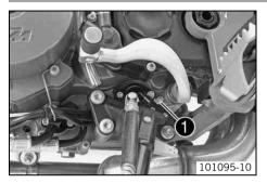
The engine number  $\bullet$  is stamped on the left side of the engine under the engine sprocket.
