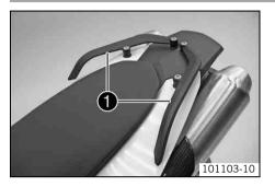
The handrails **①** are used for moving the motorcycle around. If you carry a passenger, the passenger can hold onto the handrails during the trip.
