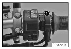
The emergency OFF switch  $\bullet$  is fitted on the right side of the handlebar.
