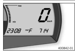
If the fuel level drops to the reserve mark, the display automatically changes to **TRIP F** and starts to count from **0.0**, regardless of the previous display mode.
