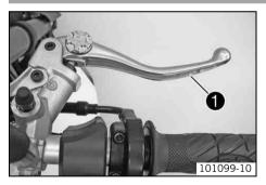
The hand brake lever  $\bullet$  is fitted on the right side of the handlebar. The front brake is engaged using the hand brake lever.
