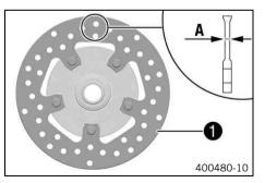
Check the thickness of the brake disc in several places to see if it conforms to measurement .
