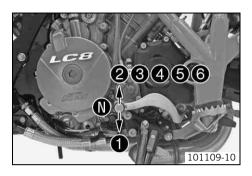
The gear positions can be seen in the photograph. The neutral or idle position  ${\bf 0}$  is between the first and second gear.
