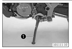
The side stand  $\bullet$  is located on the left side of the vehicle. The side stand is used to park the motorcycle.
