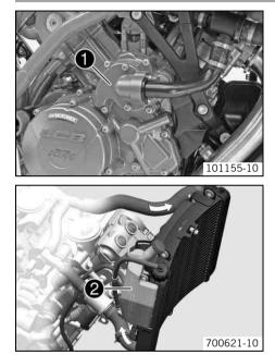
The water pump **1** in the engine forces the coolant to flow.
