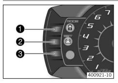
You can change the display mode with the **MODE** button ①. Possible display modes are the distance traveled (**ODO**), trip master 1 (**TRIP 1**), trip master 2 (**TRIP 2**) and the ambient temperature.
