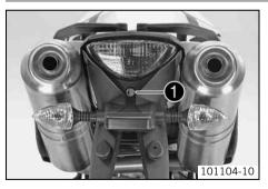
Seat lock **①** is located at the rear under the tail light. It can be locked with the ignition key.
