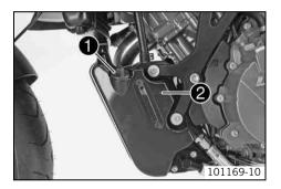
Remove plug ① and add engine oil to the top marking ②.
