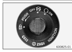
The ignition/steering lock is in front of the upper triple clamp.
